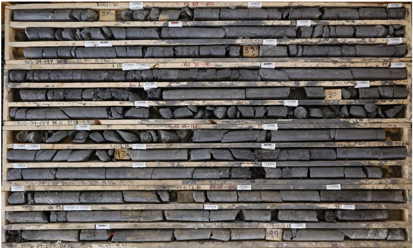
Figure 2: Core photo of KLS-24-037 between 83.84 m and 99.47 m showing intense graphite mineralization in the Loki Zone. KLS-24-037 was drilled approximately 100 m southwest of KS-CC16-12 which included a sample grading up to 22.2 % Cg (graphite), as reported in the Company’s news release on February 20, 2024.
